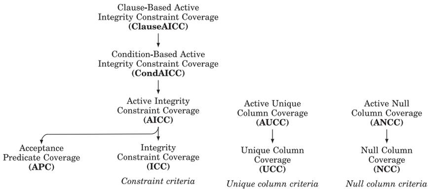
Fig. 11. The coverage criteria subsumption hierarchy for testing relational database schemas.
