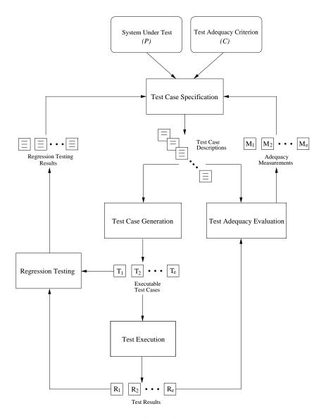
Figure 2: A Model of the Software Testing Process.
