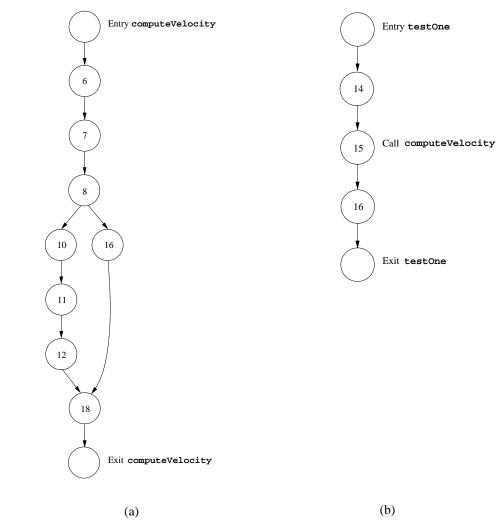
Figure 5: The Control Flow Graphs for the computeVelocity and testOne methods.
