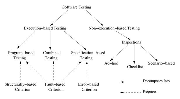
Figure 1: Hierarchy of Software Testing Techniques.
